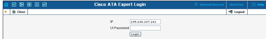
**NOTE:** The PortaBilling ATA Expert needs to communicate directly with the Cisco ATA. So make sure that the ATA is connected to the network and configured with an IP address. This IP address must be either a public IP address (accessible from anywhere on the Internet) or a private IP address (e.g. 192.168.xxx.xxx) which is accessible from the PortaBilling web server.
